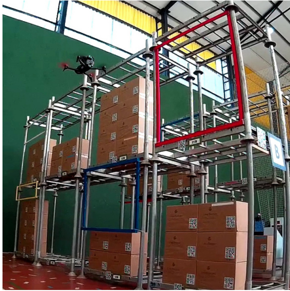
Fig. 1. Warehouse inspection using drones was the main theme in the IMAV 2019 indoors competition. In this work we describe our lightweight solution consisting of an autonomous MAV with full onboard processing, capable of self-localization using a metric monocular SLAM, and QR detection and decoding using a side inspection camera.
