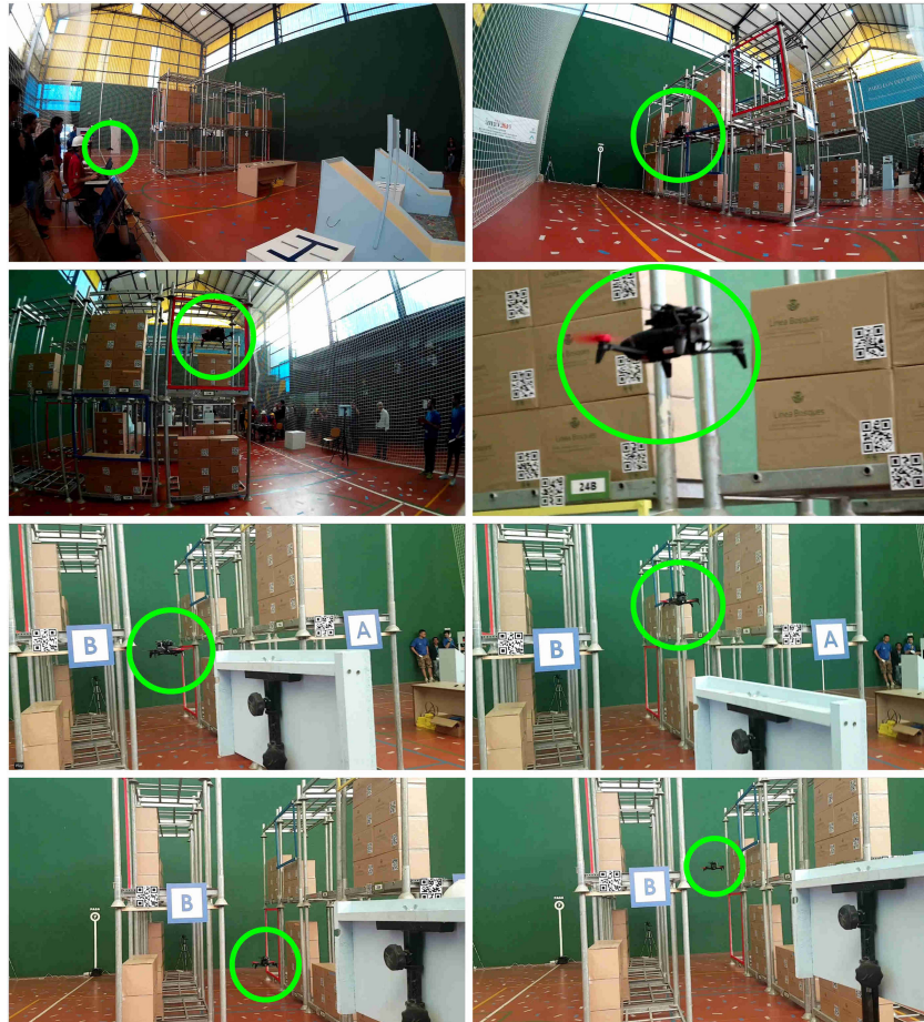
Fig. 13. Snapshots of our MAV performing autonomous flight to carry out the warehouse inspection flight. The order is from left to right, top to bottom. In the first image, the MAV takes off and flies towards rack B, and after inspecting it, it flies towards rack A, flying in between the racks to continue with the inspection, the MAV is indicated with a green circle. A video of this performance can be watched at https://youtu.be/vyOIlXkq9KA .
