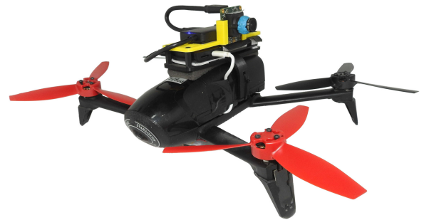
Fig. 4. Side view of the Bebop carrying the Intel Computer Stick m3 and uEye Camera.
