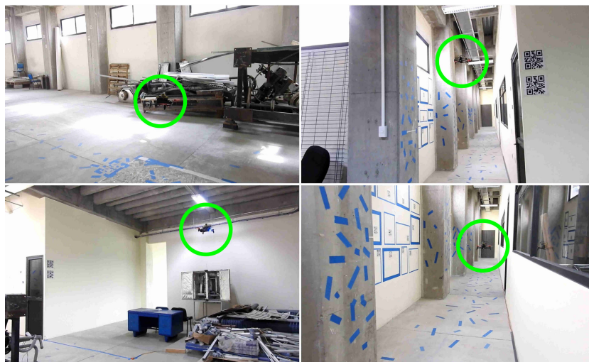
Fig. 8. External views of the MAV performing autonomous flight and inspection of the corridor in the test facility, the MAV is indicated with a green circle. A video of these experiments can be watched at https://youtu.be/vyOiIXkq9KA .
