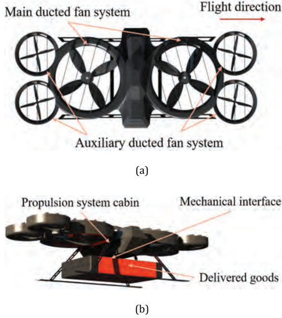
Fig. 1. The diagram of the UDAV. (a) The aerodynamic layout of UDAV. (b) The connection between UDAV and delivery goods.
