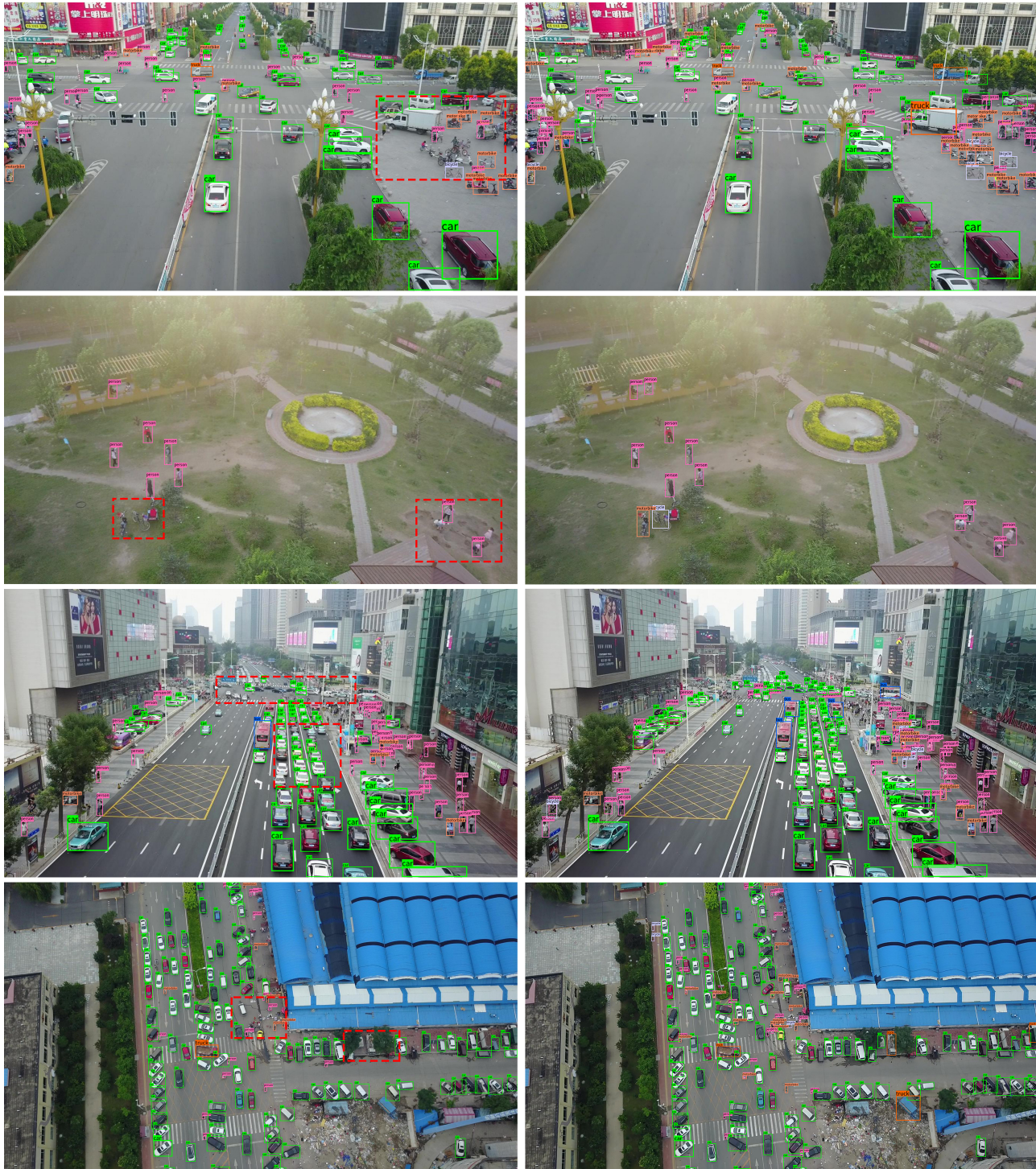
Fig. 6. Comparison of detection results by YOLOv3 (left) and PA-YOLOv3 (right) on VisDrone2018. The objects not detected by YOLOv3 are drawn in the red dotted box.
