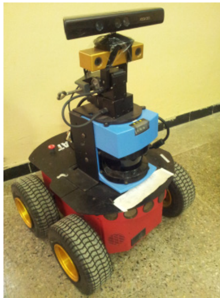
Fig. 17. The mobile pioneer robot with a mounted Microsoft Kinect camera.
