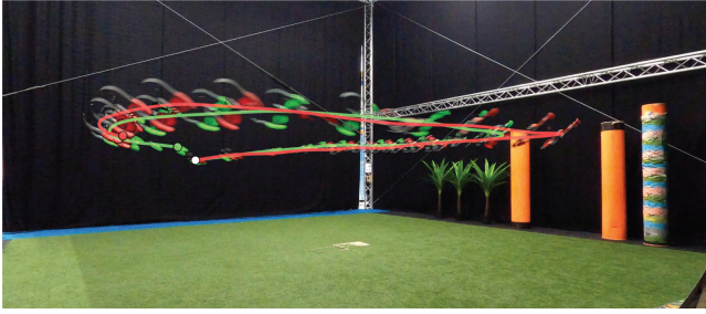
Fig. 1. A comparison of a circular flight path between the proposed controller (green) and a classical PID controller (red).
