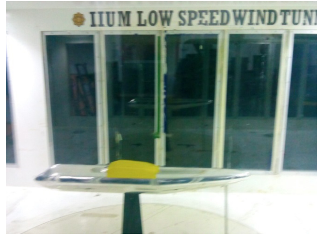
Fig. 5. Generic model of a transport aircraft.
