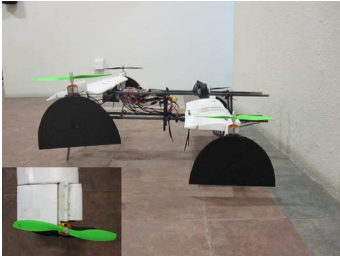
Fig. 53. Conventional setup with no tiltable wing tips.
