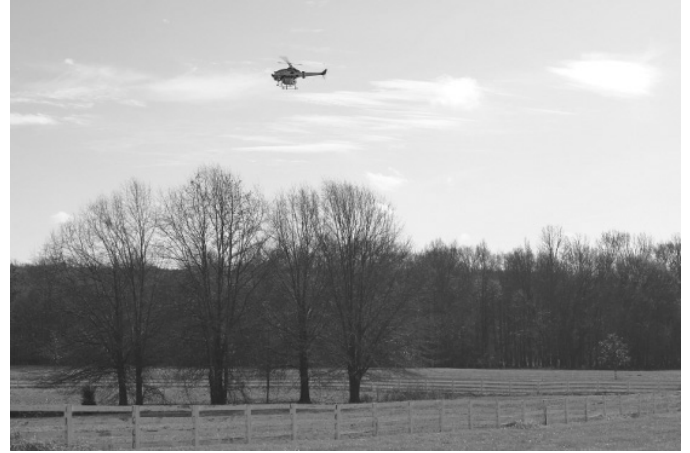
Fig. 18. (Color online) Video scene capture of the UAV test-bed successfully avoiding a tree obstacle during flight test.
