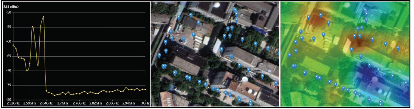
Fig. 10. Schematic illustration: (left) the power spectrum of a certain sensor, (mid) illustration of the locations of some sensors and (right) REM construction results of a specific area.
