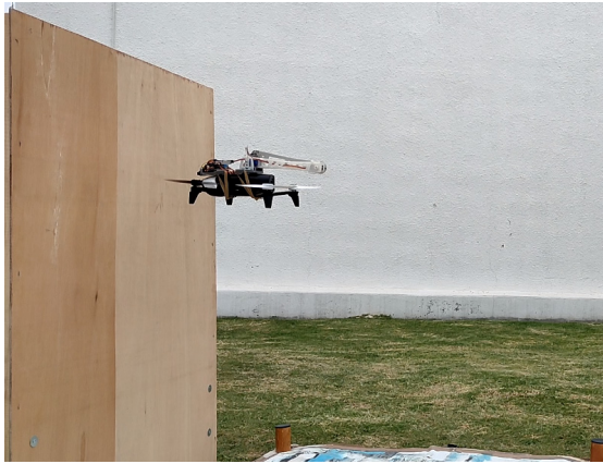
Fig. 15. Aerial manipulator near to a vertical surface. Video of experiments in the following URL: https://youtu.be/La4L8RlafE .
