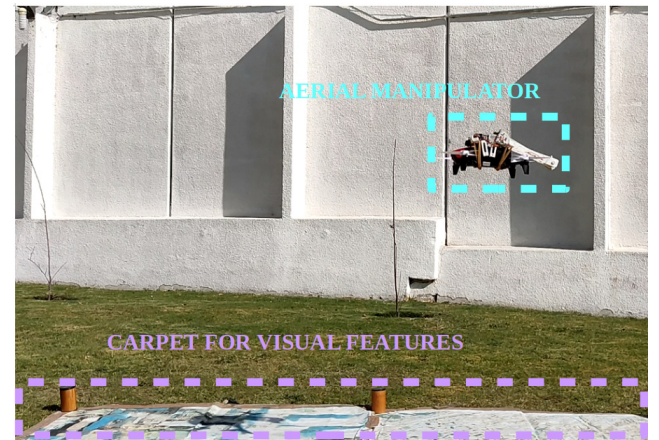
Fig. 9. Outdoor scenario. A carpet is set in the ground to provide more texture for the SLAM technique and improve the pose estimation.
