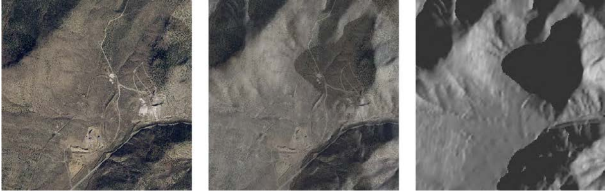
Fig. 3. Orthoimagery (left), orthoimagery with the lighting map overlaid (middle), and the lighting map \Lambda(z) (right) for one of our test areas. The lighting map was computed at 8:20 a.m. on September 15, 2011, near Eureka, UT.
