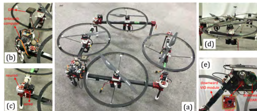
Fig. 16. (a) Main UAV prototype, (b) the upper connection part, (c) the joint part and its servo motor, (d) the tilt rotors and (e) the lower connection part [62].
