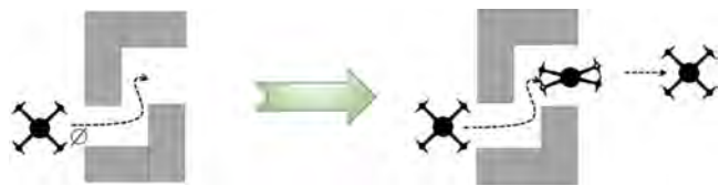
Fig. 25. Illustration of a flight scenario through a narrow place by changing the morphology of the quadrotor [38].
