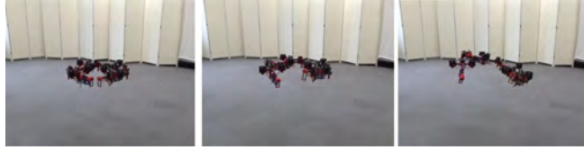
Fig. 15. Multi-link multirotor in different configurations [58].
