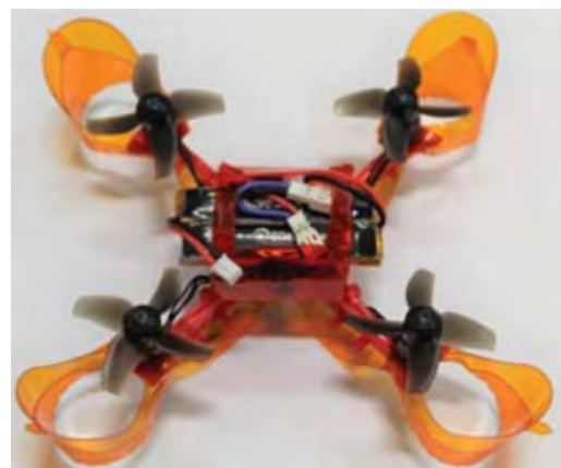
Fig. 28. Foldable quadrotor for collision resilience [41].
