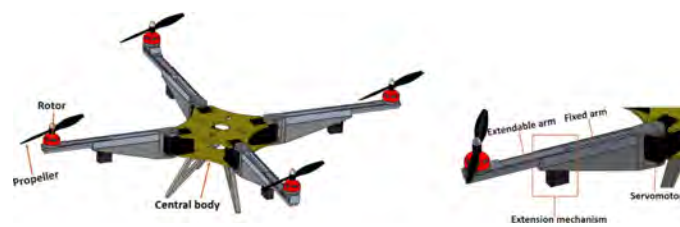
Fig. 48. Quadcopter with rotating and extendable arms [11].
