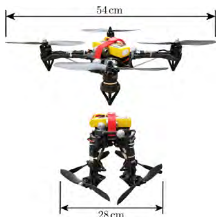
Fig. 26. Foldable quadrotor without additional actuators [39].
