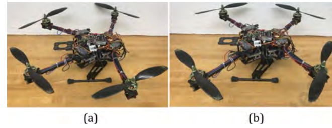
Fig. 21. Quadrotor with rotating arms: (a) optimal configuration; (b) conventional configuration [40].
