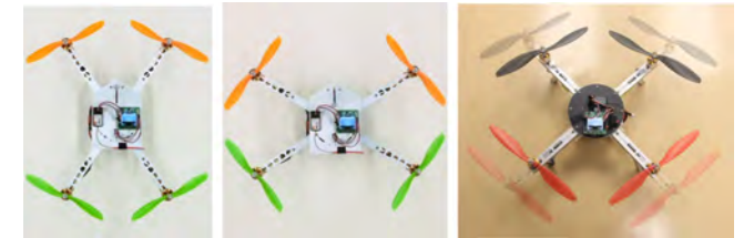
Fig. 43. Transformable quadrotors: on the left with rotating arms; on the right with extended arms [28].
