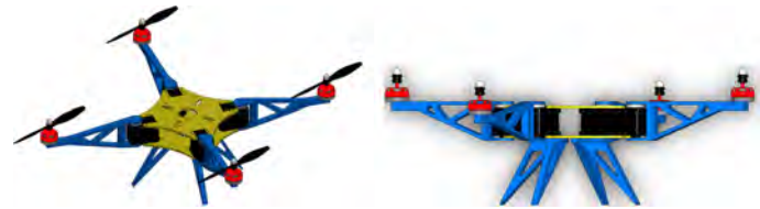
Fig. 23. Quadrotor with horizontally rotating arms [9, 20].
