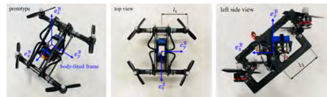
Fig. 63. Quadcopter prototype with different views, isometric, top view and left side view, respectively, [50].
