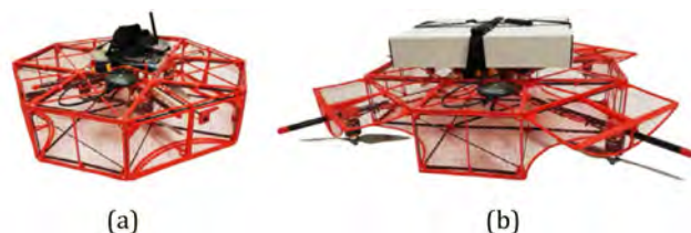
Fig. 46. (a) Drone with retracted arms. (b) Drone with extended arms [32].
