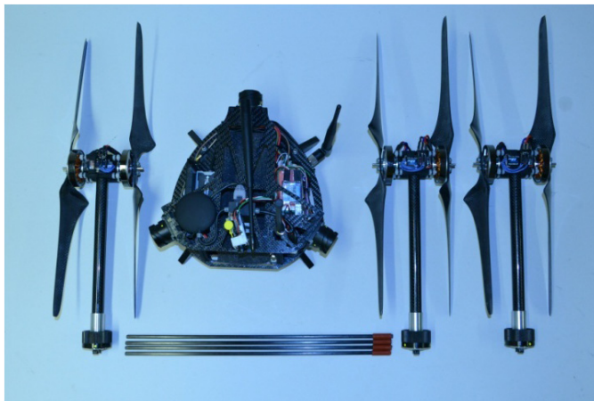
Fig. 7. HALO UAV showing detachable elements.
