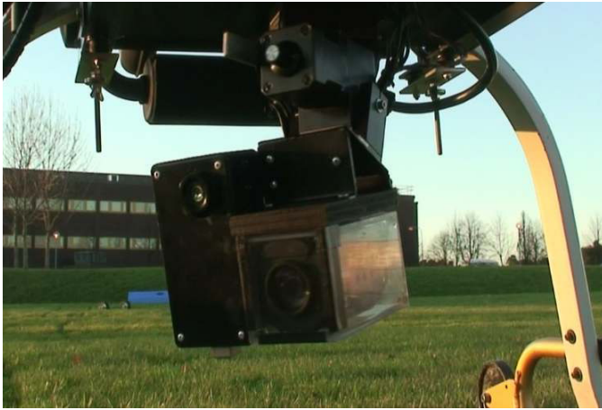
Fig. 2. On-board camera system mounted on a pan-tilt unit.
