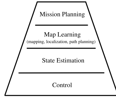
Fig. 2. Navigation stack. This figure shows the required tasks to accomplish navigation. Each level relies on information received from the next higher level.
