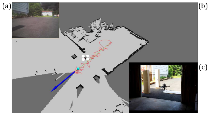
Fig. 16. Autonomous entry and exit in a real-world experiment. This figure shows the experiment at the moment that the quadrotor returns home. (a) Onboard camera view. (b) The developed 2D map, path, and trajectory. (c) Ground view of the quadrotor, exiting through the door.
